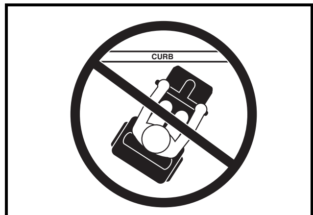
Figure 3A. Incorrect Curb Approach
